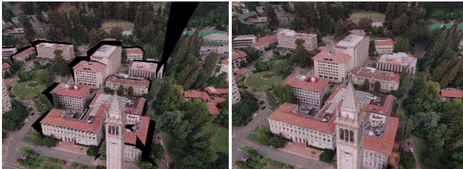
Fig. 5. The image on the left has some black regions which are invisible to all the cameras. The image on the right shows the rendering result with all the holes filled. See also Fig. 9.
